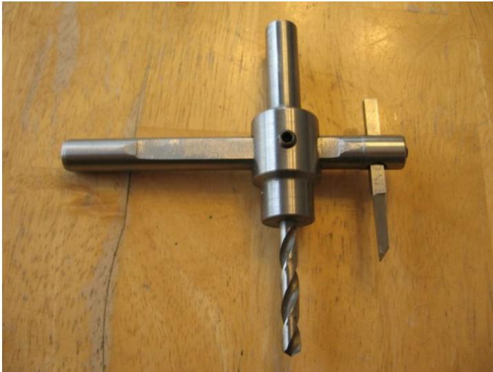
*This is a tank cutter (or trepanning) tool. It cuts only downwards, never sideways, and is used to cut holes in sheet materials. The point on the cutting tool can be toward the inside or outside depending on whether you want to keep the disc cut out (on the inside, as here) or the material surrounding the disc.*
