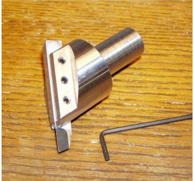
*This is a fly cutter tool. It is most often used cutting sideways for flat surface facing operations. It is never used cutting downwards to cut holes. However, model engineers often use it cutting downwards to cut curved surfaces such as on a smokebox saddle or the under-side of a chimney.*
